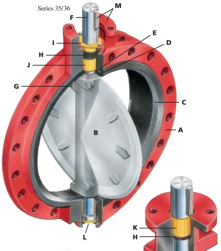
**SECONDARY SEAL** (**E**) A secondary seal is achieved by an interference fit of the stem and seat hole diameters.
